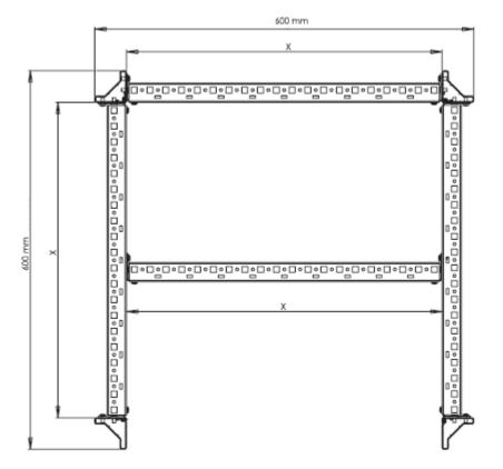
In terms of both width and interior depth size, TEOS body structure is designed at the same coefficient rate. The complete structure inside the body is designed at the 25mm coefficient. Thus, the width rail can also be installed on the depth rail.
