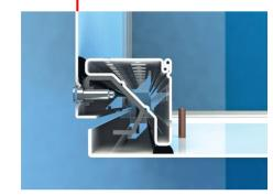
All gaskets apply pressure on the convex frame curves. Dust and water particles are left in the space between the convex curves, and thus pressure on the gasket is prevented.
