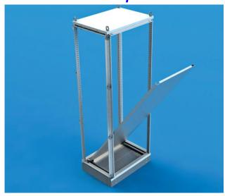
Manufactured from galvanized steel, TEOS plus+ mounting plates are railed and easily mounted. With its thick steel sheet structure, the mounting plate can carry heavy equipment with its rigid structure and does not need additional side support parts. In this way, bayed enclosure space is increased in combined enclosures.
